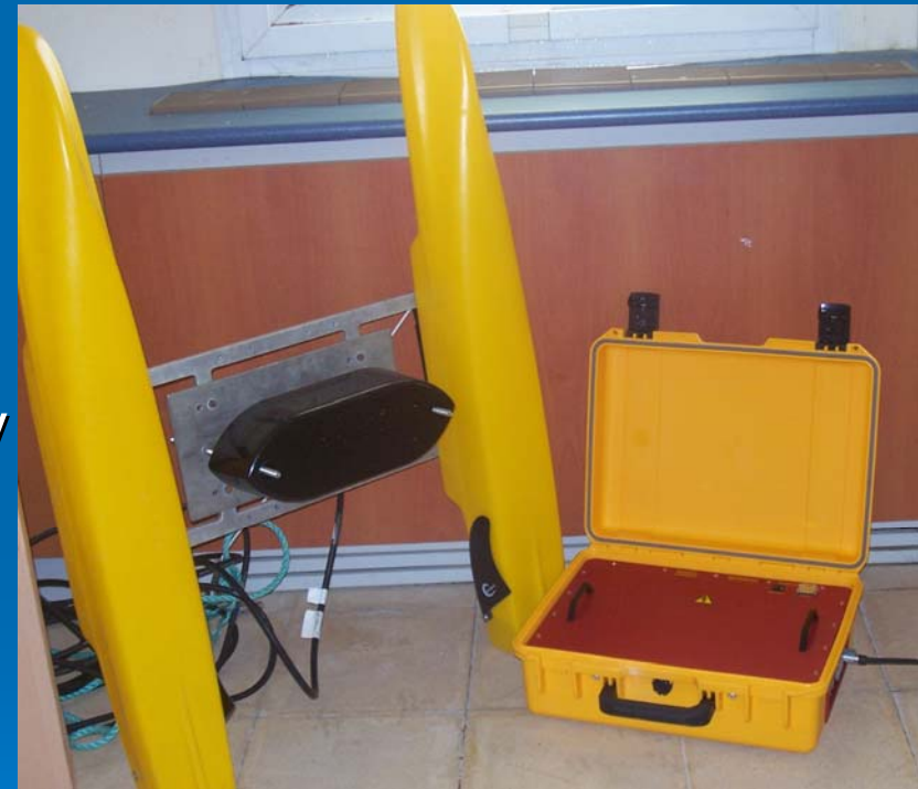
320 B/P dual frequency echo sounding system (by Knudsen Engineering)
