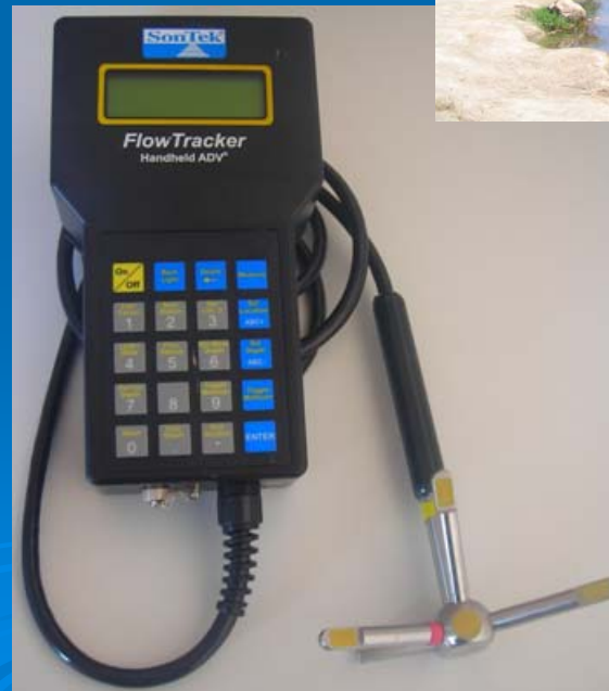
Acoustic Doppler Velocimeter (ADV) Flowtracker (10,000 kHz)
